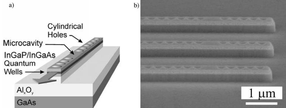
Figure 7. a) Schematic of 1-D PBG microcavity laser structure. The line of cylindrical holes forming the photonic crystal provides strong optical confinement along the waveguide. b) A SEM micrograph showing several completed microlaser structures.
