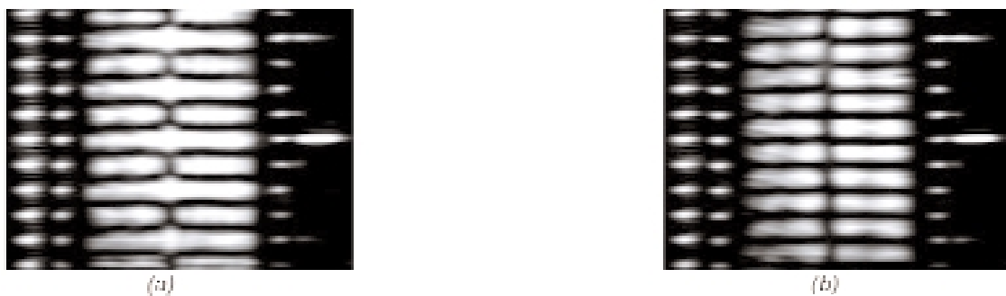
Fig. 12: (a) Aligned position: Spatial phase matched between bar-bar, fringe-bar, and fringe-fringe. (b) Misaligned position: fringes aligned, bars apparently aligned, but fringe-bar phase shift of 180 deg. indicates 1-fringe-cycle misalignment.
