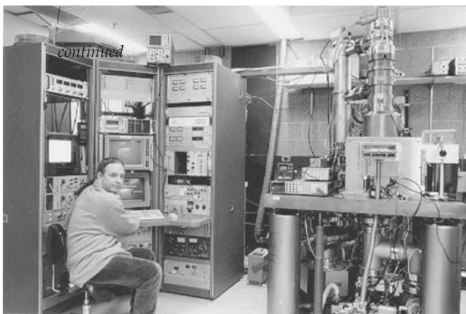
Fig. 3: Photograph of the VS-2A scanning-electron-beam lithography system. The operator is Research Specialist Mark Mondol.
