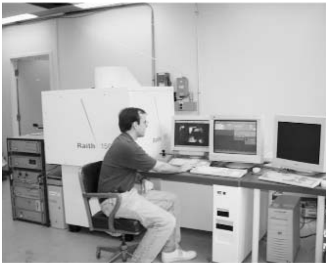
Fig. 3: The Raith-150 electron-beam lithography system. This tool provides sub-20-nm patterning resolution, and will be used to demonstrate nanometer pattern-placement accuracy via spatial phase locking. The operator is graduate student J. Todd Hastings.
