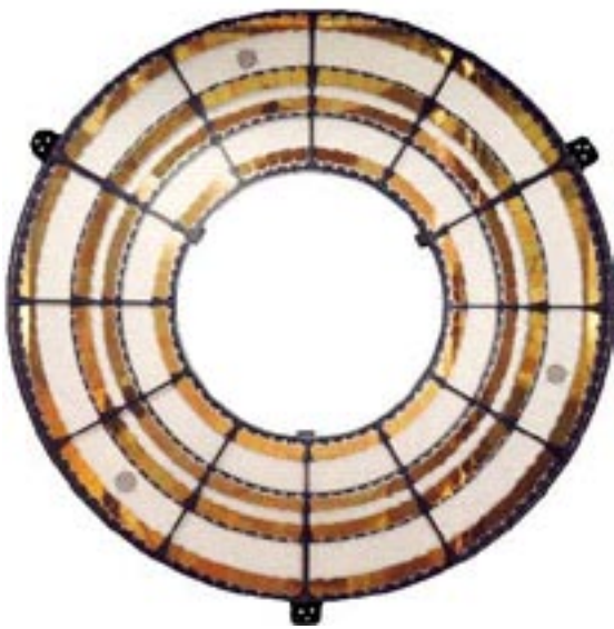
Fig. 13: Photograph of the HETGS flight instrument on the Chandra X-ray telescope, which consists a 1.0 meter-diameter aluminum wheel populated with hundreds of 200 nm and 400 nm-period gold X-ray transmission gratings (340 total).
