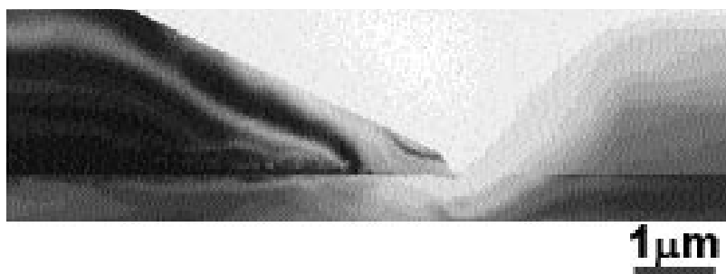
Fig. 5: Cross sectional TEM micrograph of 1\ \mu\text{m} of Ge selectively grown on Si.
