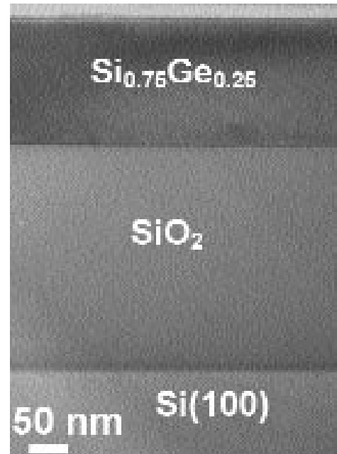
Fig. 1: Cross-sectional TEM of the SiGe on oxide structure fabricated using wafer bonding and tech-back.
