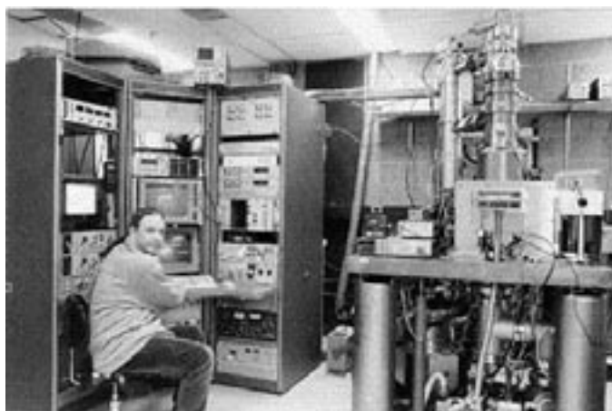
Fig. 7: Photograph of the VS-2A Scanning-Electron-Beam Lithography System (SEBL). The operator is Research Specialist Mark Mondol.
