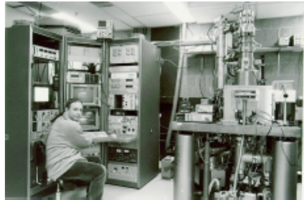
Fig. 4: Photograph of the VS-2A scanning-electron-beam lithography system. The operator is Research Specialist Mark Mondol.
