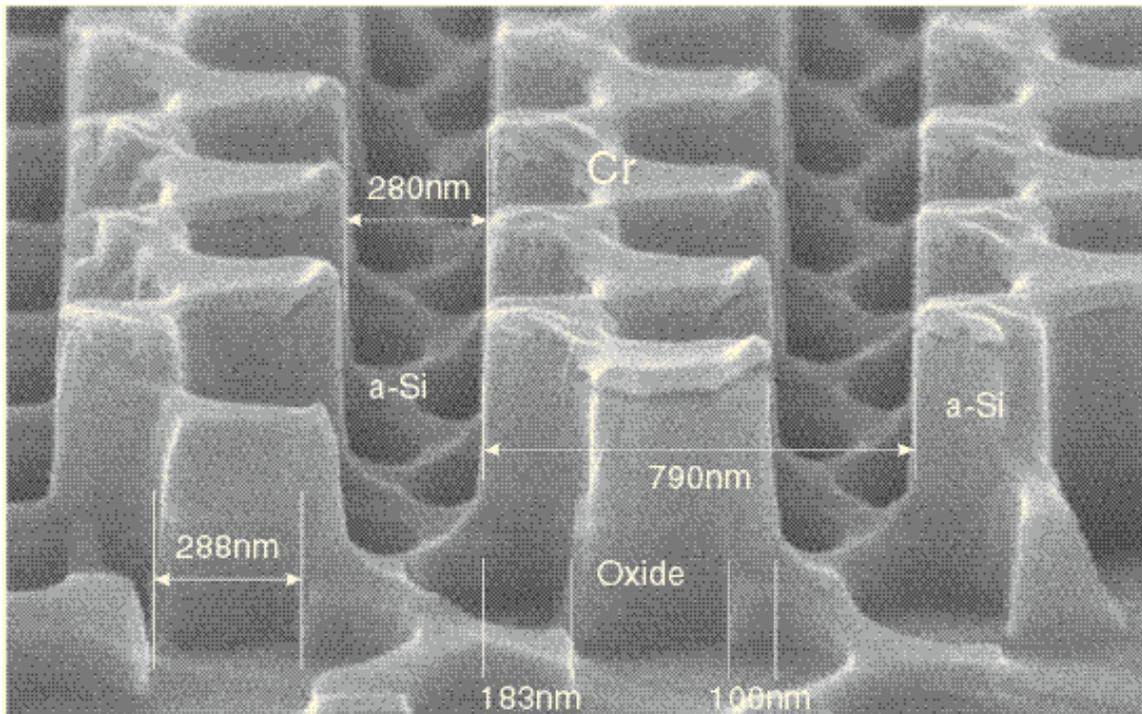
*Scanning-electron micrograph of the patterned second layer of a 3-D photonic-bandgap structure, showing amorphous Si on top of the first-layer structure, with groves filled with  $\text{SiO}_2$ . The second layer structure is shifted by half of the periods in both x and y directions. An intentional overetch into the first layer is also observable.*
