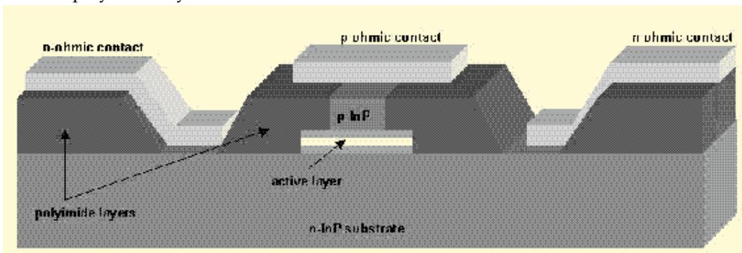
Fig. 3: Co-planar stripline laser structure.
