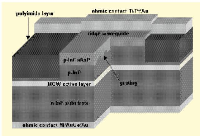
Fig. 1: Schematic of a polyimide-planarized InP DFB ridge-waveguide laser.
