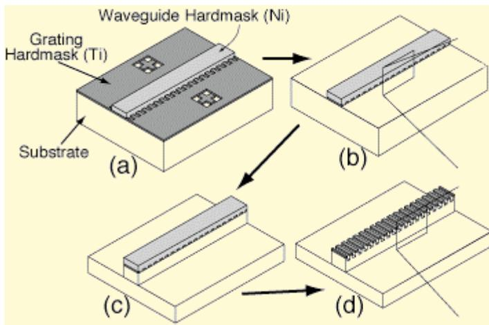
Fig. 14: The Dual-Hardmask Process is used to pattern the fine-period gratings atop the InGaAsP waveguides. (a) First the grating-level hardmask is patterned over the substrate, then the waveguide-level mask is patterned over the grating-level mask. (b) The excess grating mask is stripped. (c) The waveguide features are dry-etched. (d) After removal of the waveguide mask, the grating features are dry-etched.
