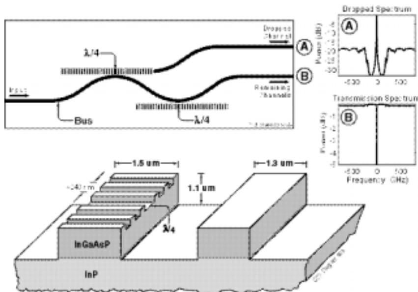
Fig. 13: Diagram of the channel-dropping filter. As depicted in the upper portion, a multi-wavelength input signal is launched along the bus waveguide. One resonant wavelength-channel is dropped in the upper port of the device. As shown in the lower portion of the Figure, the waveguide is composed of InGaAsP, surrounded by an InP cladding.
