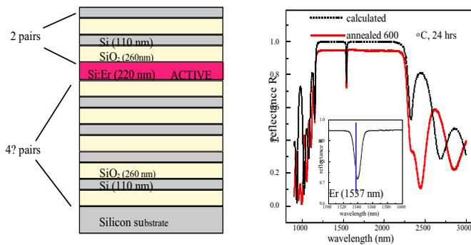
Fig. 8: (left) Si/SiO<sub>2</sub> microcavity with Si:Er active layer. The cavity has an active layer that is tuned for 1537 nm. (right) Reflectance spectrum of microcavity with resonance at 1537 nm. The cavity quality factor is ~300. (fabricated at Polaroid-Norwood).
