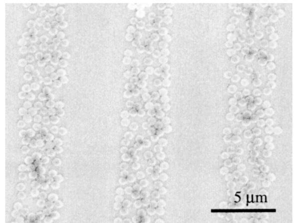
Fig. 9: SEM micrograph of SiO<sub>2</sub> spheres (diameter 0.7  $\mu\text{m}$ ) deposited on bilayers of LPEI/PAA polyelectrolyte stripes. The stripes are patterned via micrcontact printing, and have a width of 4  $\mu\text{m}$ .
