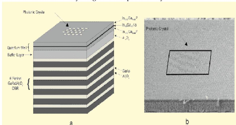
Fig. 6: a) 2-D PBG light emitting diode structure. The InGaP/InGaAs quantum well structure emits at  $\lambda = 980 \text{ nm}$ . The active region is separated from the DBR by a low refractive index  $\text{Al}_x\text{O}_y$  separation layer. This separation increases the amount of emitted light reflected from the DBR. A hexagonal lattice of holes in the top layer of the device eliminates coupling of emitted light to guided modes. b) SEM micrograph of 2-D PBG light emitting diode.
