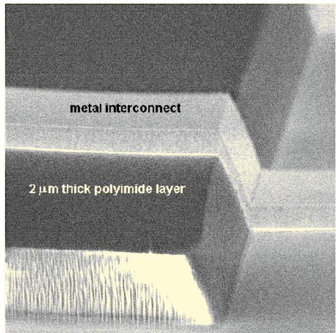
Fig. 4: Scanning electron micrograph of a low capacitance polyimide based metal interconnect.
