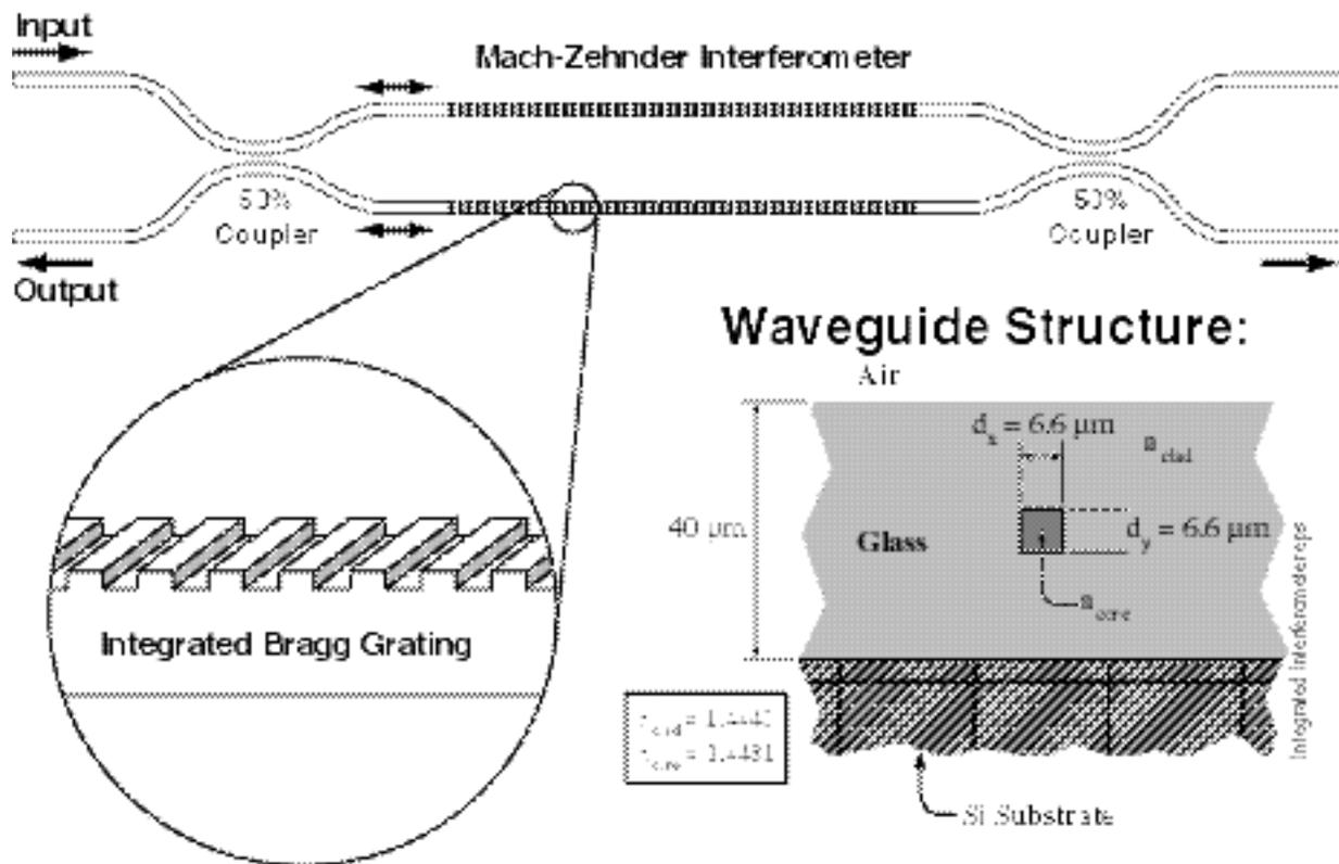
Fig. 12: Diagram of an integrated optical matched-filter. The waveguide consists of a germanium-doped  $\text{SiO}_2$  core,  $6.6 \mu\text{m}$  wide and tall, surrounded by  $\text{SiO}_2$  cladding. The 10 mm-long Bragg grating is formed by etching a shallow, 535 nm-period grating onto the top of the waveguide before the upper cladding layer is deposited. The waveguide interferometer is designed to redirect the reflected, filtered signal to a separate output port.
