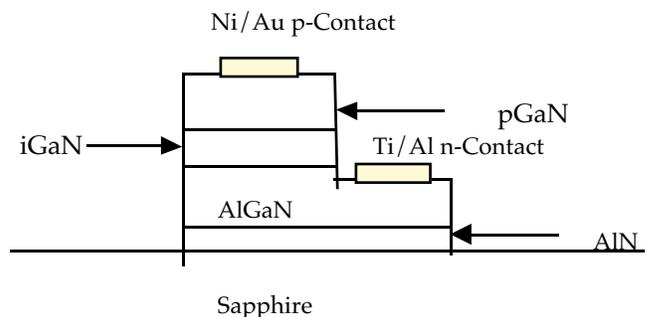
Fig. 5: Structure of the diode.
