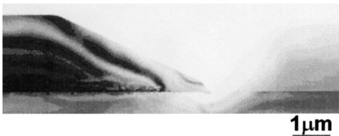
Fig. 2: Cross sectional TEM micrograph of 1mm of Ge selectively grown on Si.
