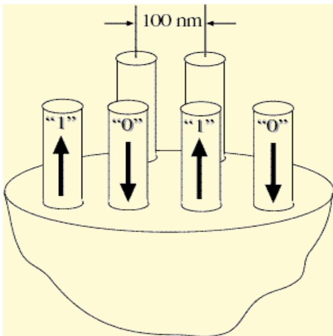
Fig. 21: Schematic of high density magnetic information storage based on sub-100 nm sized magnetic particles.
