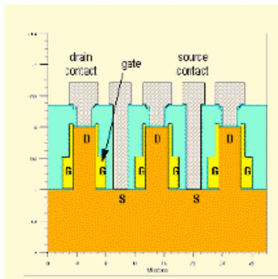
Fig. 16: VMOS Process simulation
