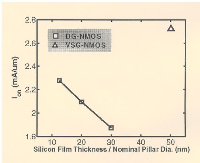
Fig. 4: Simulation results: Drive-current density for DG- and VSG-MOS designs.  $T_{ox} = 1.5$  nm,  $V_{dd} = 1$  V,  $V_{th} \sim 400$  mV. Midgap gates. Hydrodynamic models used.
