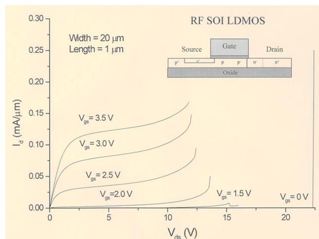
Fig. 10: Device output characteristics
