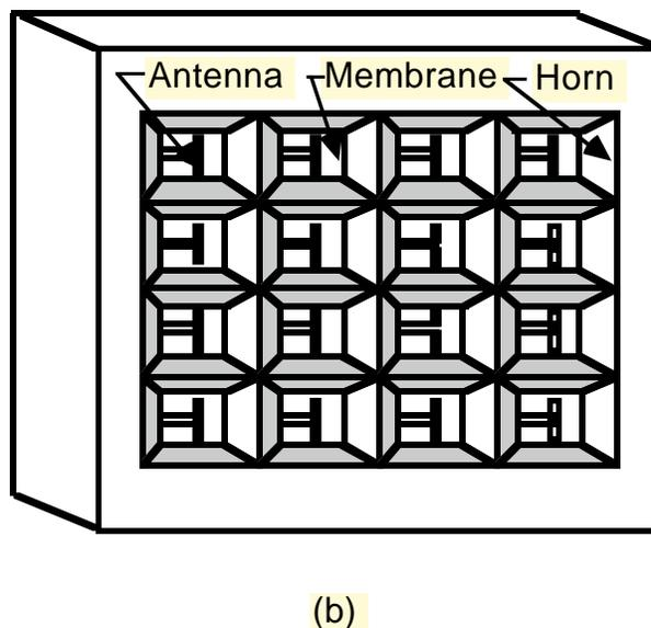
Fig. 18: (a) Example of a micromachined horn antenna structure that is made by anisotropically etching a  $\langle 100 \rangle$  silicon wafer. (b) Schematic of a focal-plane array on a single wafer made using micromachining.
