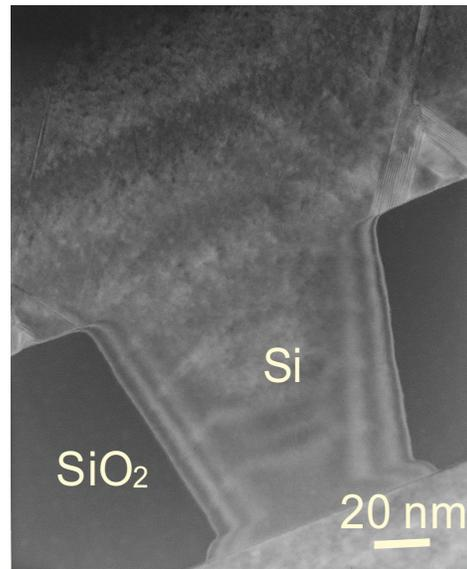
Fig. 5: TEM image of selective epitaxial filling of 100 nm holes in  $SiO_2$
