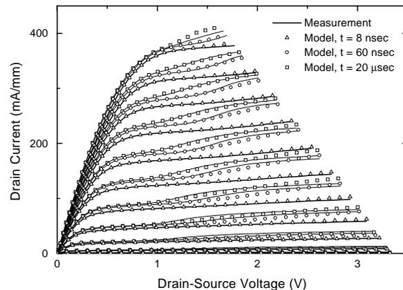
Fig. 14: Pulsed I-V characteristics of InAlAs/InGaAs HEMTs fabricated at MIT at three different times after the device is turned on. Also graphed are the predictions of a new equivalent circuit model of the kink.
