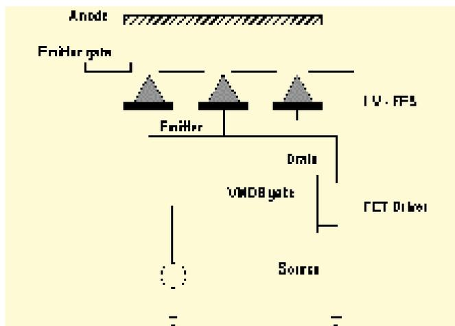
Fig. 15: MOSFET/FEA Schematic
