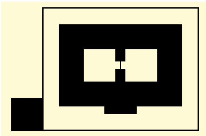
Fig. 6: Gate mask layout of a figure-eight geometry MOSFET. The inner two white square areas are the source and drain probe pads that will be salicided. The dark wide ring is the gate pad with the active gate being the fine line in the center. The outer ring is a guard ring.
