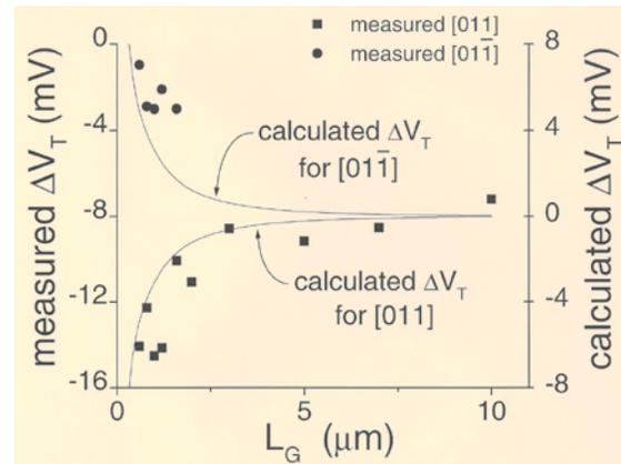
Fig. 12: The change in threshold voltage,  $\Delta V_T$ , of InP HEMTs after exposure to forming-gas (5% H<sub>2</sub> in N<sub>2</sub>) at 200°C for 3 hours. The  $L_G$  and orientation dependencies are key signatures of the piezoelectric effect, and indicate that  $\Delta V_T$  is in part due to mechanical stress. This stress arises from titanium hydride formation in the Ti/Pt/Au gate. Also shown is the predicted  $\Delta V_T$  due to a piezoelectric-induced volume charge distribution.
