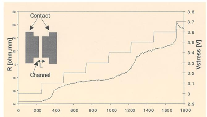
Fig.13: Time evolution of low-field resistance of a TLM with a 12  $\mu\text{m}$  long channel. The TLM is stressed at a bias  $V_{stress}$  that is stepped up from 3 to 3.7 V in 0.1 V intervals.
