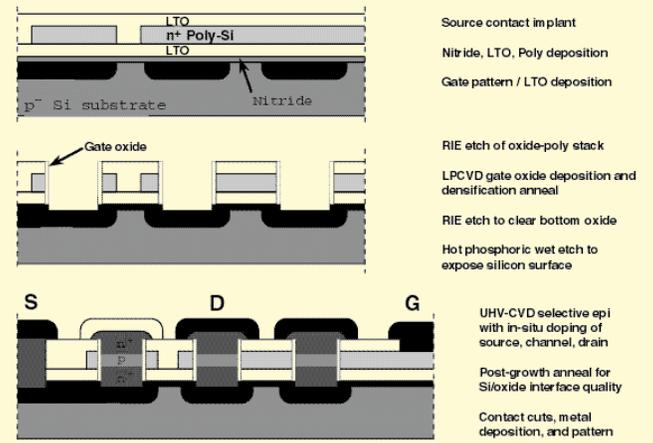
Fig. 2: Process for fabricating surround-gate vertical MOS devices.
