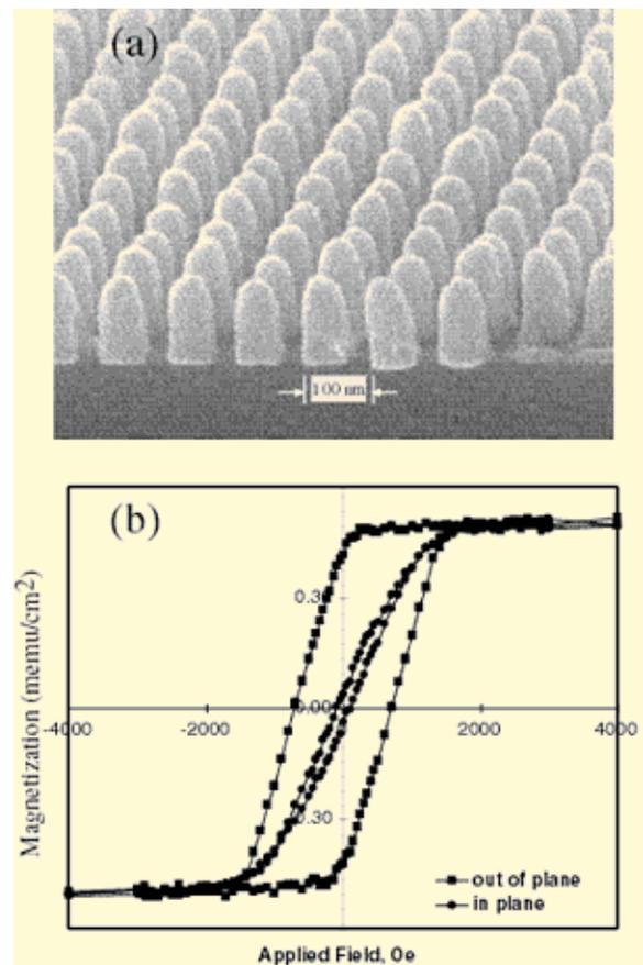
Fig. 22a: An electron micrograph of 100 nm-period Ni pillars after the removal of the ARC plating template. Figure 22b is a plot of the magnetization of the pillars vs. a magnetic field applied in-plane (dots) and out-of-plane (squares). The large magnetization at remanence (applied field = 0) for the out-of-plane compared to the in-plane applied field indicates that out-of-plane magnetization is favored.
