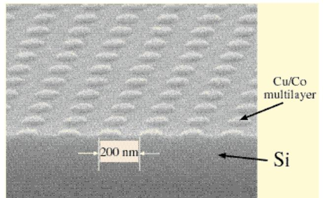
Fig. 26: 200 nm-period islands of Cu/Co multilayers, patterned by interferometric lithography and ion milling, are suitable for magnetic random access memory (MRAM) applications.
