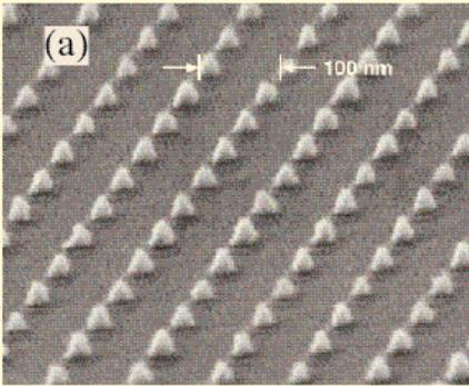
Fig. 25a: Evaporated NiCr pyramids after lift-off. (b) In-plane (dots) and out-of-plane (squares) magnetization curves obtained by Superconducting Quantum Interference Device (SQUID) magnetometry at 10 K of a similar Ni sample. Such pyramids, whose magnetization is unstable at room temperature, also favor out-of-plane magnetization at 10 K.
