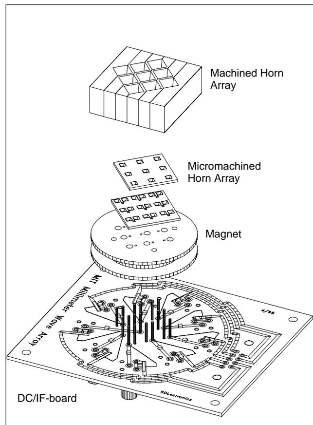
*Schematic of an array structure including a micromachined and machined horn array, the device wafer, and the dc and IF connection board. (b) I-V curves of seven SIS junctions in the array. (Courtesy of Q. Hu)*
