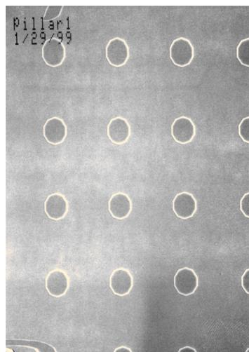
Fig. 17: Vertically etched Si pillar arrays (top view)
