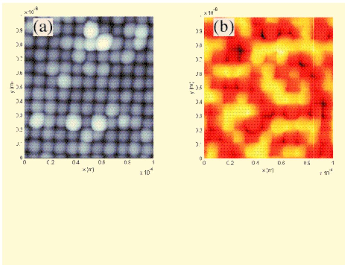
Fig. 24a: Topography plot of the electroplated Ni pillars obtained by scanning the pillars with the tip of a magnetic force microscope and recording tip deflections. Figure 24b is the corresponding magnetic-force plot where the light regions indicate “up” magnetization and the dark regions indicate “down” magnetization.
