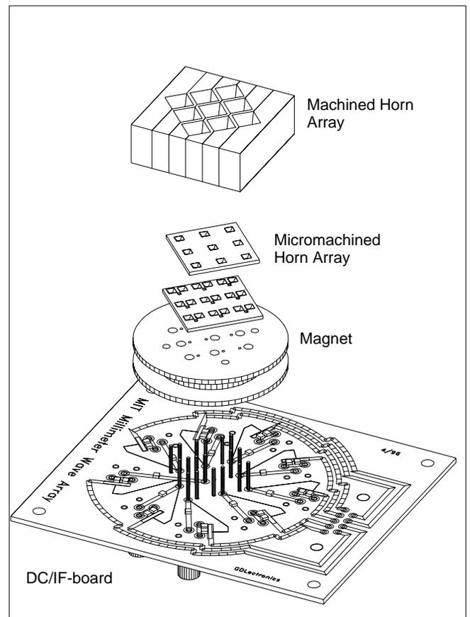
Fig. 19: (a) Schematic of an array structure including a micromachined and machined horn array, the device wafer, and the dc and IF connection board. (b) I-V curves of seven SIS junctions in the array.
