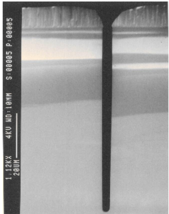
Fig. 11: 84- $\mu\text{m}$  deep, 5- $\mu\text{m}$  wide via etched in silicon using the Deep Reactive Ion Etcher (DRIE)
