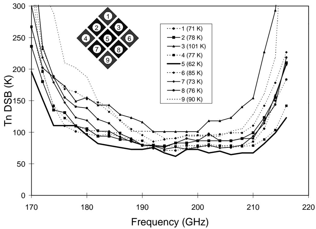
Fig. 20: Measured DSB noise temperatures of all the nine elements in the array. The inset shows the minimum noise temperature for each individual element.
