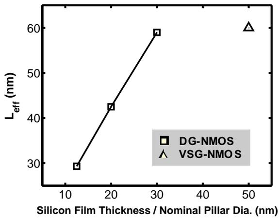
Fig. 3: Simulation results: Minimum acceptable  $L_{eff}$  (for  $I_{off} = 1 \times 10^{-8}$  A/mm) for DG- and VSG-MOS designs.  $T_{ox} = 1.5$  nm,  $V_{dd} = 1$  V,  $V_{th} \sim 400$  mV. Midgap gates.
