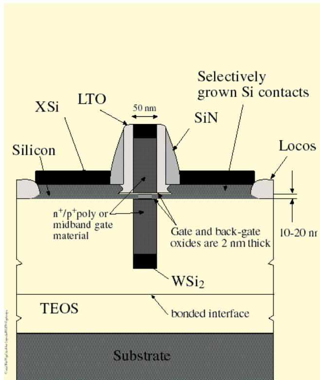
Fig. 1: Double-gate NMOS transistor with 25 nm effective channel length. Gate-to-gate alignment is via IBBI.
