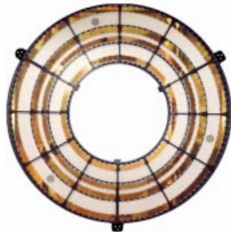
Fig. 29: Photograph of the HETGS flight instrument, which consists of a 1.0 meter-diameter aluminum wheel populated with hundreds of 200 nm and 400 nm-period gold X-ray transmission gratings (340 total).
