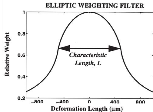
Fig. 4: 1-D cross-section of an elliptic weighting filter. The characteristic length is defined as the section length when the relative weight has dropped to  $2/\pi$ . The filter shape corresponds to the deformation profile of an elastic material under distributed load in a circle of radius  $L/2$ .
