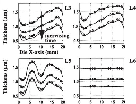
Fig. 6: Model prediction for “up” areas polished under process a for different times. The elliptic weighting filter length is 3.80 mm.
