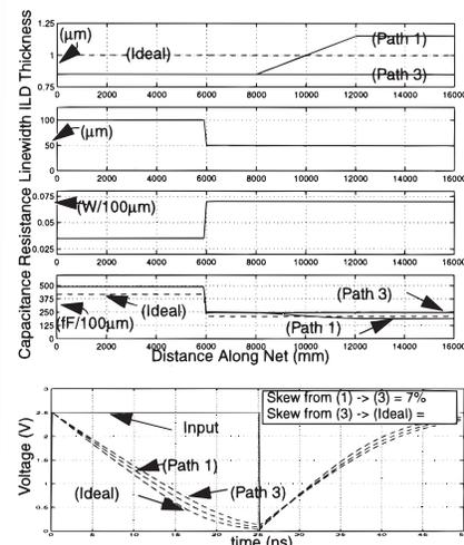
Fig. 8: Resulting ILD thickness and capacitance along clock paths (top); resulting clock skews (below).
