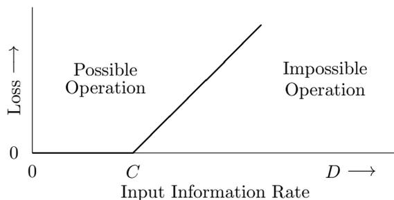
Figure 6.4: Channel Loss Diagram. For an input data rate  $D$ , either less than or greater than the channel capacity  $C$ , the minimum possible rate at which information is lost is the greater of 0 and  $D - C$
