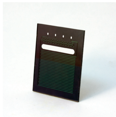
FIGURE 1: Silicon microreactor with 400\text{-}\mu\text{m} -wide channels. The top half of the reactor is cooled and thermally isolated from the heated bottom half.
