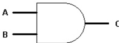
Figure 7.2: Circuit diagram of an AND gate
